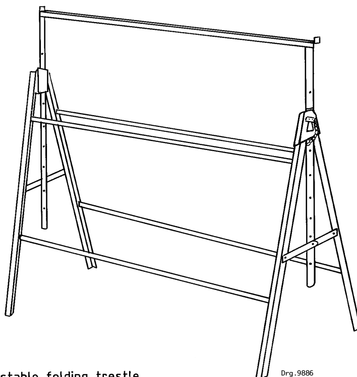
(b) Adjustable folding trestle (steel type)
